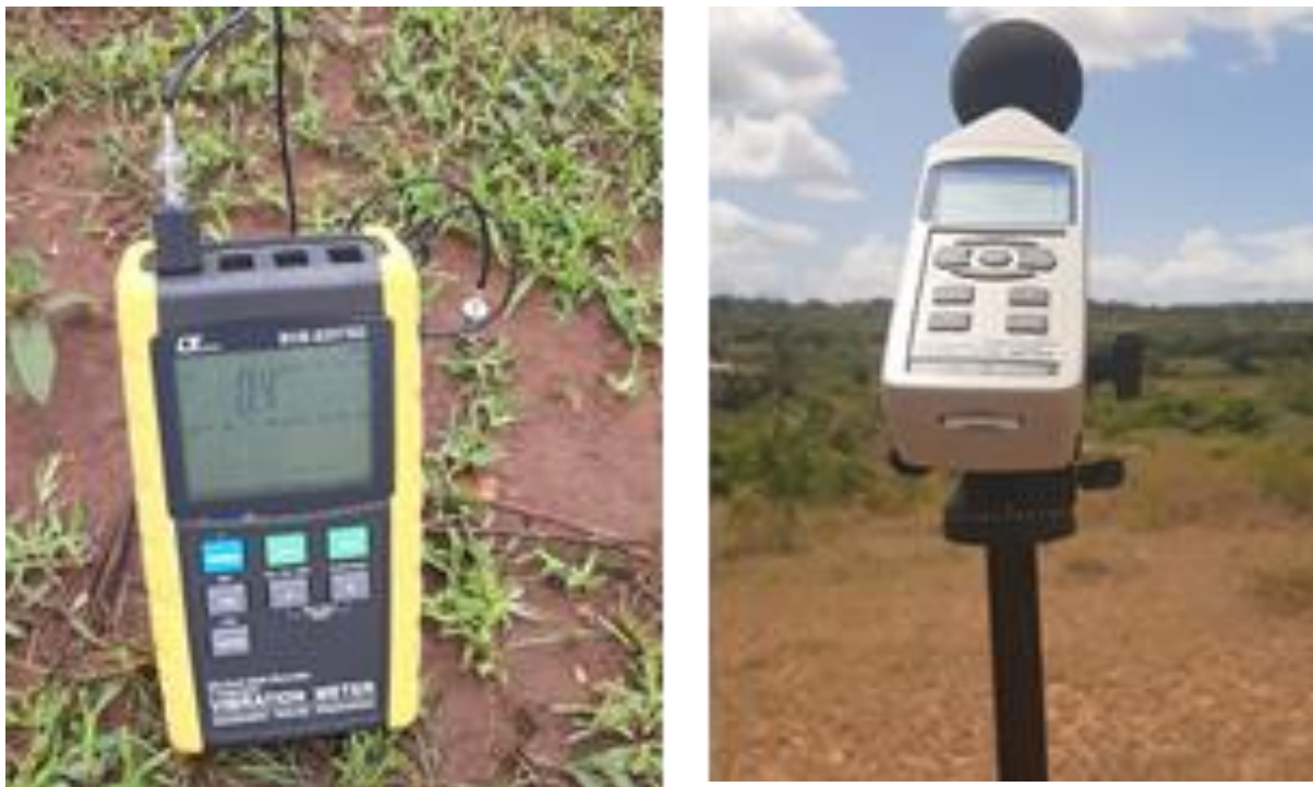
Figure 4-11: Noise and vibration level meters used to collected data on the project site
